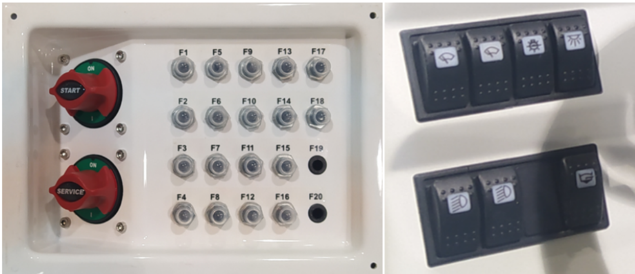
Figure 5. Location of switchboard and fuses
